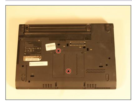
• Remove the two J00 screws on the backside.
