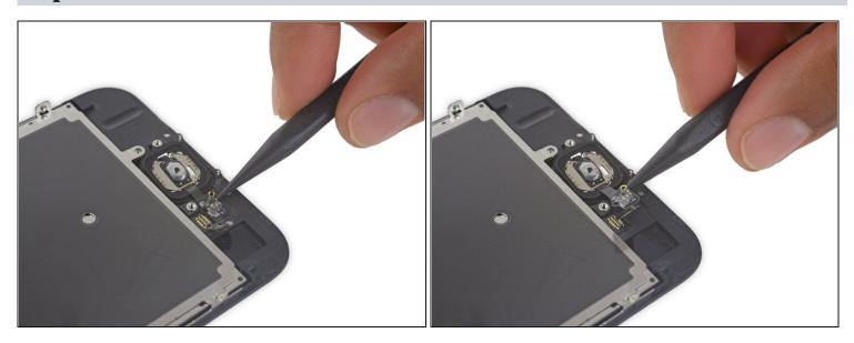
• Use the pointed tip of a spudger to carefully separate the home button flex cable from the back of the display panel.
