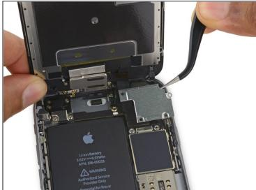
• Remove the display cable bracket.
