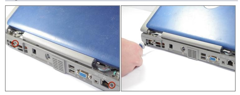
• Remove two screws (5.8mm) located behind the screen.
