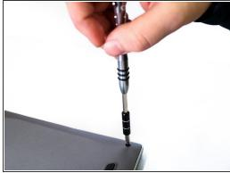
Flip over the Lapdock and remove the four 3.5mm long phillips head screws from the bottom.
