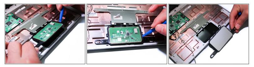
Unplug track pad from the ribbon cable that is attaching it to the motherboard then use a plastic prying tool to take out the track-pad.
