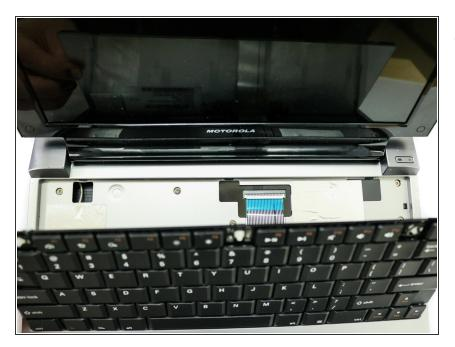
Lift up keyboard so that you are able to see the ribbon cable connected to the contact.
