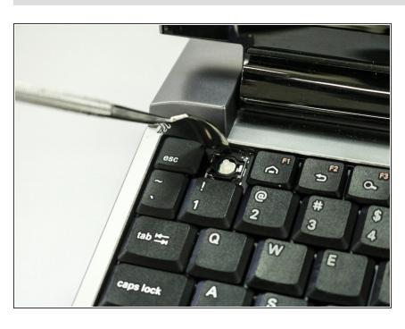
You can use a small metal spudger to depress each tab to avoid scratching the keyboard.
