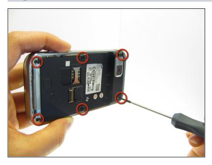
Remove six (4.28 x 1.25)mm screws using the Phillips #00 screwdriver
