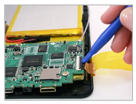
Use a plastic opening tool to push back the ZIF connector to release the ribbon wire on the motherboard.
