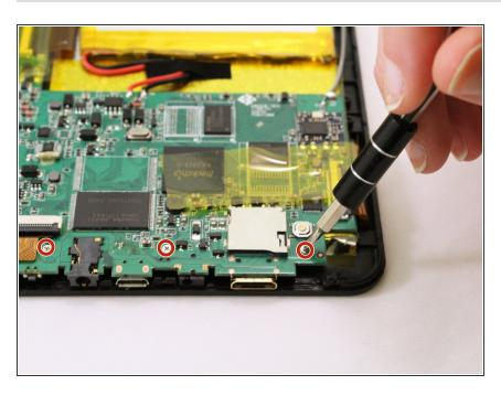
Remove three 4 mm screws from the motherboard.
