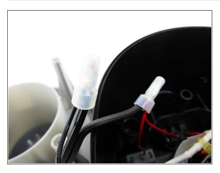
Remove plastic coverings and aluminum wrap to unattach the power cord.
