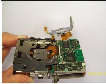
Carefully lift the shutter along with the ribbon connected to it. This will remove the casing around the motherboard.
