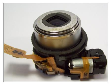
Once you have removed the lens from the main chassis, gently brush off any dirt, sand, or dust that may have accumulated in the crevices.
