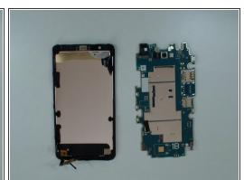
Remove the logic board.
