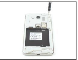
• Remove the nine 4mm screws screws from the midframe with a Phillips #000 screwdriver.
