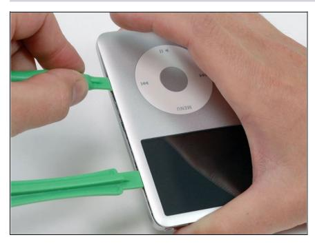
Remove the opening tool from the top corner and insert it into the seam between the front and back of the iPod, leaving at least 1.5 inches of space between the two tools (as done on the other side).
