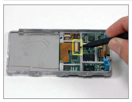
Use a spudger to flip up the plastic tab holding the orange display ribbon in place. The tab will rotate up 90 degrees towards the display, releasing the ribbon cable.
