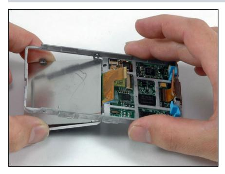
Lift the framework assembly up, and slide the display and LCD metal backplate out of the framework assembly.
