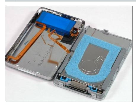
Place the rear panel next to the iPod, being careful not to strain the orange headphone jack cable.
