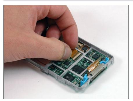
Slide the orange display ribbon cable directly out of its connector.
