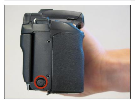
Remove the plastic remote control socket cap by pulling it straight out.
