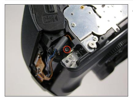
Remove one 4.8 mm silver screw securing Remote Control Socket to camera.
