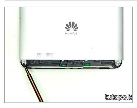
• Unscrew the two screws on the left and right of the case.
