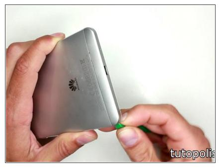
Remove the case tab on the bottom of the phone with a spudger or a pick.
