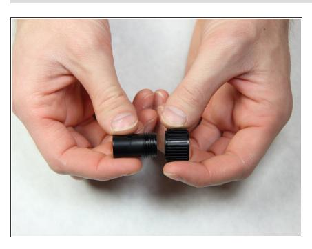
Separate the lens and the gear by unscrewing the gear.
