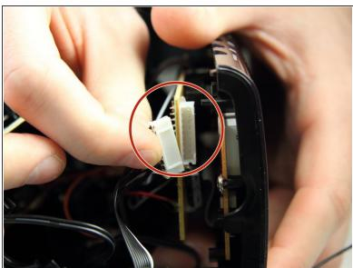
Unplug the projector's connector from the circuit board.
