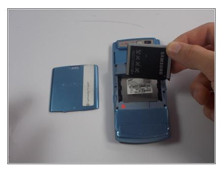
Remove the old battery and replace with the new one.
