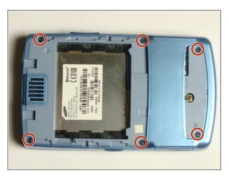
Locate the six screws and remove them with a Phillips #00 Screwdriver.
