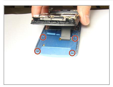
Locate and remove the four screws with a Phillips #00 Screwdriver.
