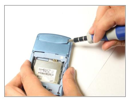
Use a flat-head screwdriver to remove the back lid.
