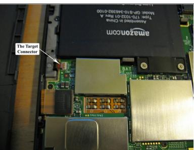
Here is the flex connector that will be soldering to. The other side is closer to the external connector, however there is very little room between it and one of the RFI shields.
