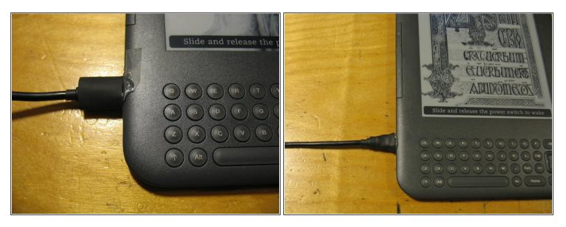
Some more heat shrink and trimming the hot glue should result in a nice finish.
