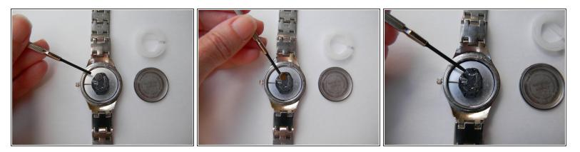
• Take the old battery out of the watch. You can use the mini flat head screwdriver to do this.
