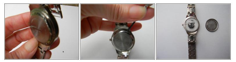
• You will need to take the back of the watch off. To do this you will turn the watch over to the back side and look carefully for a small groove opening. This is where you will use the mini flat head screwdriver. Insert the flat head screwdriver into the groove and pop the back off of the watch.
