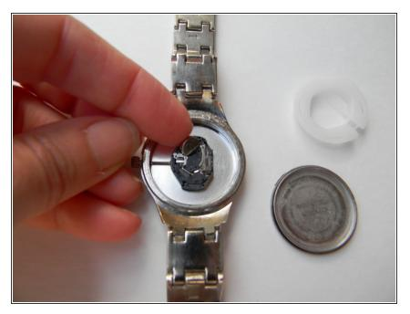
Put the new battery in watch. Use your fingers to insert the new battery.
