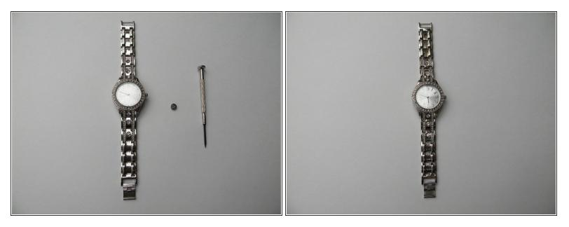
• For this project you will need the watch you are replacing the battery on, the new battery and a mini flat head screwdriver.
