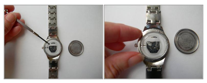
• Take the white plastic ring out of the watch. You can use the mini flat head screwdriver or your finger to pull it out.
