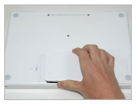
Lift the hatch, and remove it from the laptop
