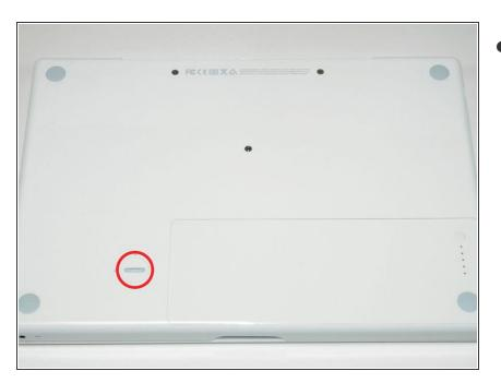
Rotate the battery latch 90° in clockwise with a coin.
