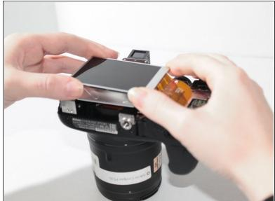
Lift the LCD screen upwards.
