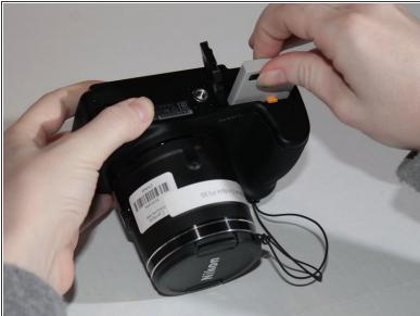
Gently remove the battery from the chamber.
