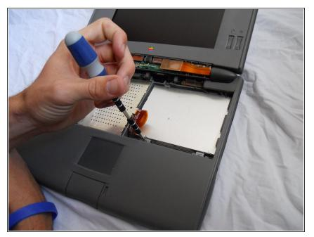
Remove the three T8 Torx screws securing the floppy drive to the frame.
