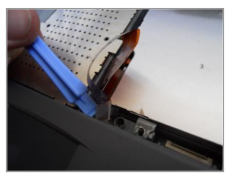
Using a spudger, lift the plastic tabs on the floppy drive securing the ribbon cable to the ribbon port.
