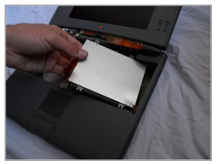
• Lift the defective floppy drive from the body of the computer.
