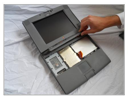
• Remove the plastic panel at the bottom of the display.
