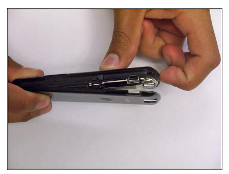
Remove the phone back cover by pushing down on the black tab located at the top center of the Motorola Phone.
