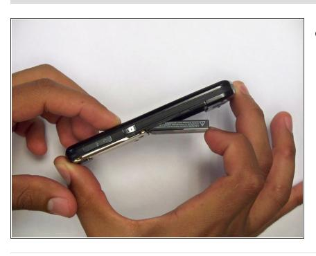
Remove the battery by pulling the battery from the top center.
