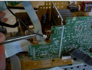
Disconnect the black wire by gripping the wire at the base and pulling gently until released.
