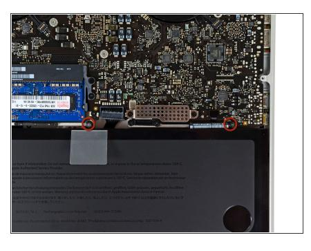
Remove the two 7.4 mm Tri-point screws securing the battery to the upper case.
