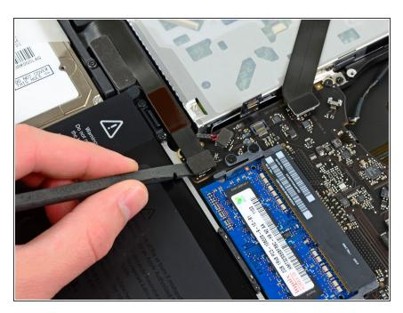
Disconnect the hard drive/IR sensor cable from its socket on the logic board by lifting up from beneath its connector.
