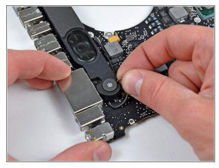
i If necessary, lift the microphone out of its recess in the left speaker housing.
