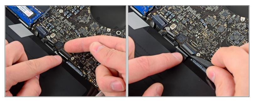
Use your fingernail to flip up the retaining flap on the keyboard ribbon cable ZIF socket.
