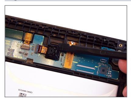
Use the spudger to remove the main body of the camera from the rest of the device. This should be done anywhere around the black-framed perimeter of the camera.
