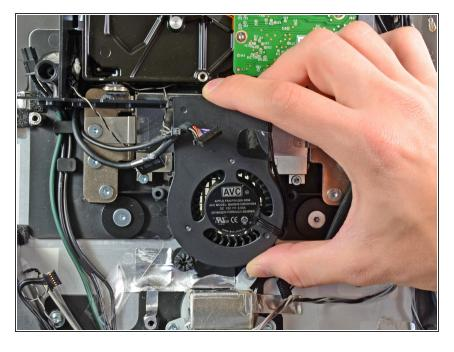
Pull the hard drive fan away from the back of the outer case and remove it from the iMac.
