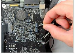
Disconnect the microphone, left speaker, and right speaker cables by pulling their connectors toward the right side of the iMac.
