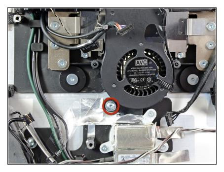
Remove the single 13 mm T10 Torx screw securing the hard drive fan to the outer case.
