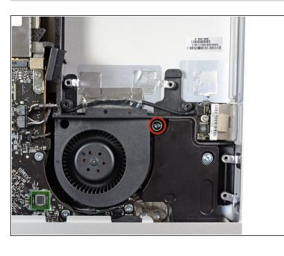
Remove the single 13 mm T10 Torx screw securing the optical drive fan to the outer case.
