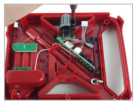
Remove the two 1 cm Philips #0 screws that secure the tuning dial panel to the device case.
