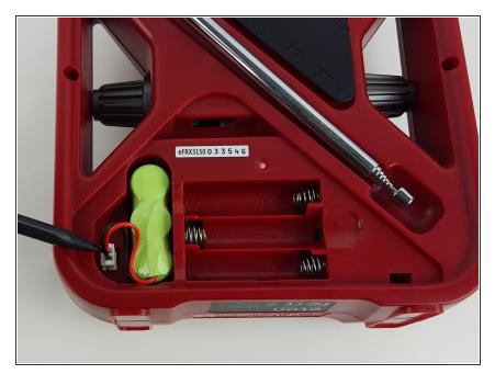
• Disconnect the battery pack wires from the device and remove the battery pack.
