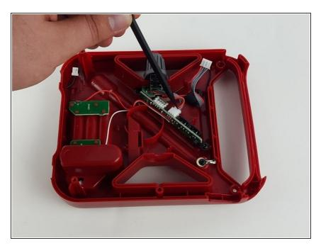
Unplug the socket connection from the I/O board as shown in the image.
