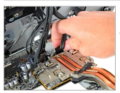
Being careful not to damage the socket on the logic board, gently pull the hard drive SATA data cable straight out of its socket on the logic board.
