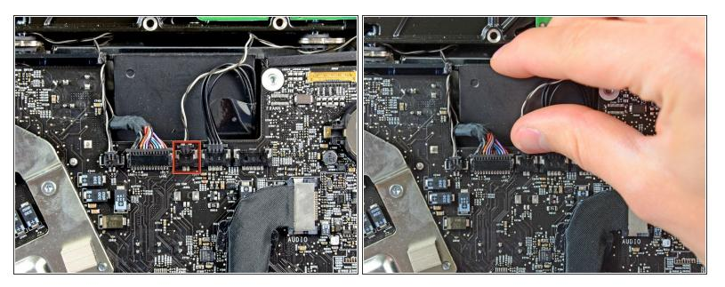
Pull the optical drive thermal sensor connector straight up from its socket on the logic board. Pull parallel to the board.
