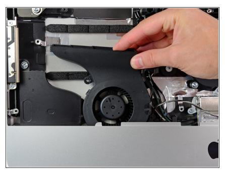
• Pull the CPU fan straight up from its mounting pin near the bottom edge of the iMac.
