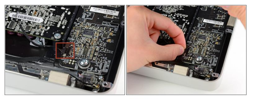
Pull the vertical sync cable connector out of its socket on the LED driver board near the top left corner of your iMac.
