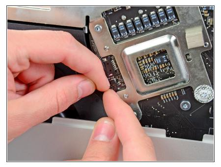
Pull the power button connector toward the bottom left corner of the iMac to disconnect it from its socket on the logic board.
