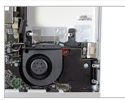
Remove the single 13 mm T10 Torx screw securing the optical drive fan to the outer case.
