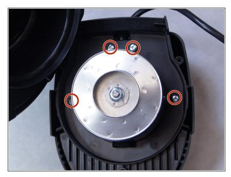
Use a 3.5 mm hex key to remove the four screws securing the power unit assembly.
