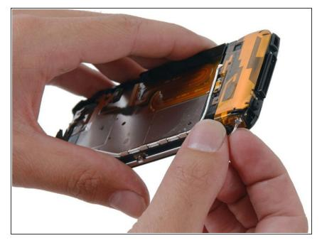
• Disconnect the antenna cable to the left of the dock connector.
