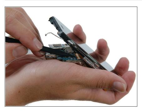
• Flip up the retaining bar to free the dock connector cable.
