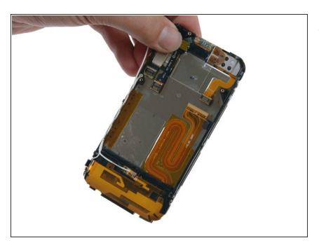
• View of the iPhone with the logic board and battery removed.
