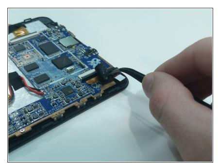
Using tweezers, carefully remove the cloth covering from the ribbon connector for the camera.
