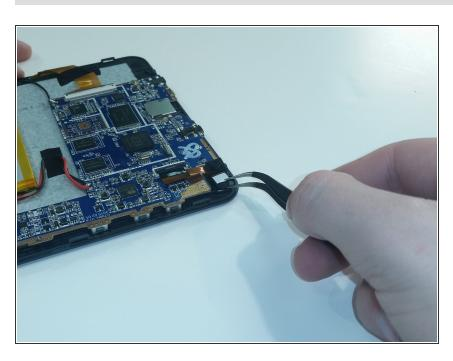
Remove the camera from its position at the top of the tablet.
