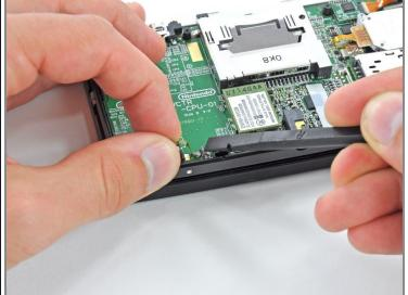
• Use the flat end of a spudger or your fingernail to flip up the retaining flap on the Microphone ribbon cable ZIF socket.
