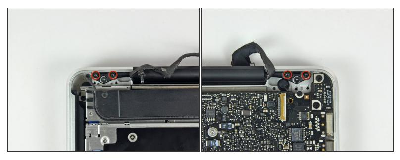
Use your Torx driver to remove the two outer 6.5 mm screws securing each of the two display brackets to the upper case (4 screws total).
