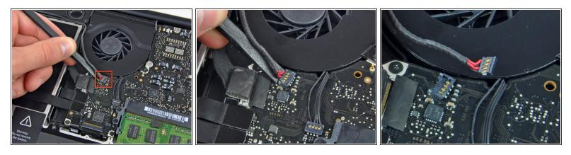
Use the flat end of a spudger to pry the subwoofer/right speaker cable connector up off its socket on the logic board.
