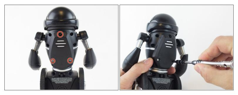
• Remove the three 12.0 mm Phillips # 2 screws from the battery cover.
