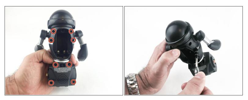
Remove the eight 9.3 mm Phillips #1 screws from the back of the robot.
