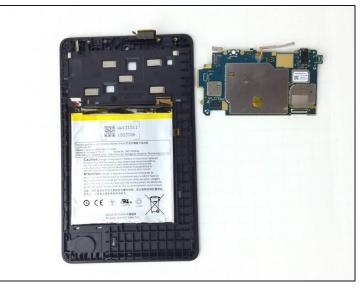
• Position the iFixit Opening Tool beneath the motherboard and pull upwards to remove the motherboard from its case.
