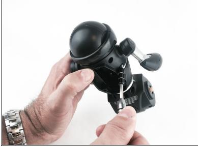
Remove the eight 9.3 mm Phillips #1 screws from the back of the robot.
