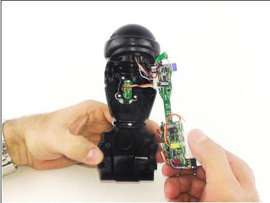
Carefully pull the motor and motherboard assembly straight out from the base.
