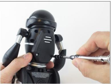
Remove the three 12.0 mm Phillips # 2 screws from the battery cover.
