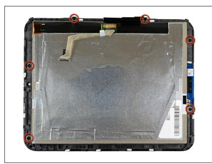
Remove the six 2.2 mm Phillips screws securing the LCD to the front panel.
