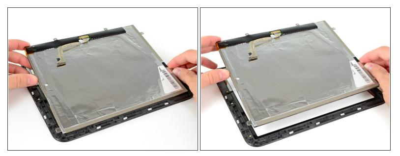
• Lift up the LCD assembly and remove it from the front panel.
