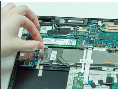
Using the flat end of the spudger, pry the edge of the ribbon wire on top of the memory card so it is loose enough to detach from the memory card.
