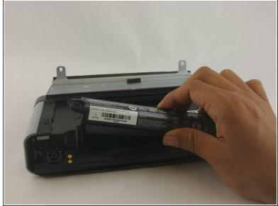
Remove the two 12.5 mm Phillips #2 screws from the sides of the battery.
