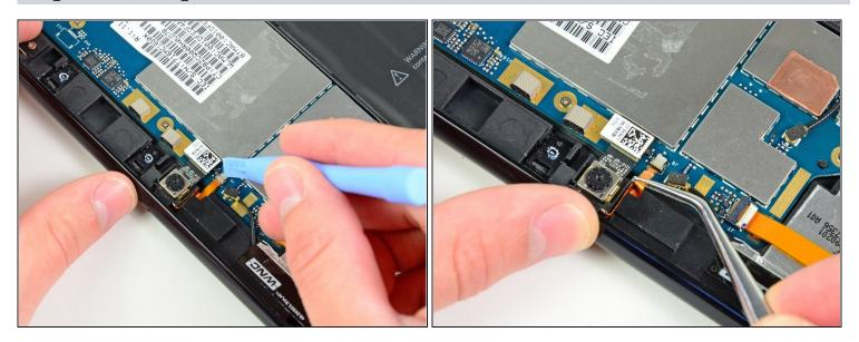
• Use the edge of a plastic opening tool to flip up the microphone ribbon cable retaining flap.
