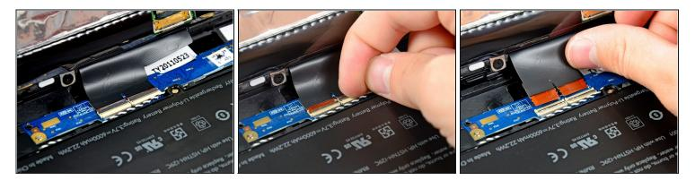
• Use your fingernail to carefully flip up the retaining flaps on the two digitizer ribbon cable ZIF sockets.
