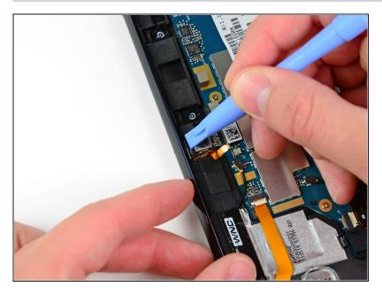
• Use the edge of a plastic opening tool to pry the microphone away from the portion of the rear case right above the camera.
