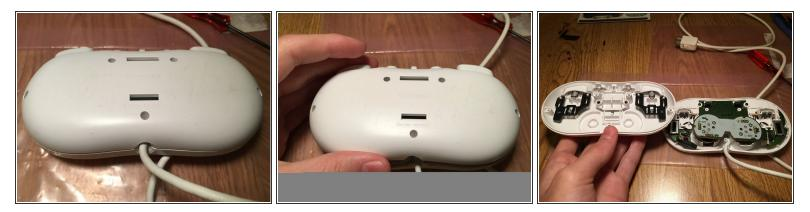
• Upon removal of triwing screws, the rear panel assembly should lift right off.
