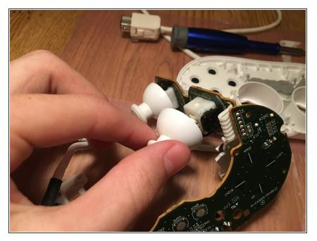
The analog stick covers just pull straight off from the stick on the logic board.
