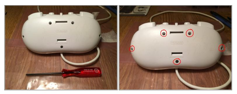
• First things first: remove the 5 triwing screws on the back. Ensure you have a proper triwing screwdriver, as a Phillips or flathead screwdriver will strip the screw pretty easily.
