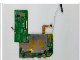
Remove the motherboard by lifting from the area indicated
