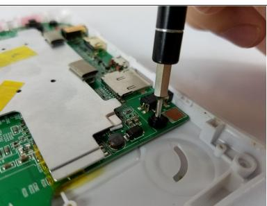
Remove the seven 4 mm Phillips #000 screws with a PH#000 screwdriver
