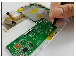
Remove the tape that is attaching the motherboard to the plastic casing
