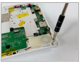
Using a Phillips PH 000 screwdriver, unscrew the two 3 mm Phillips #000 screws on each side of the speakers that hold the speakers in place.
