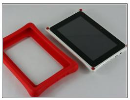
Remove the rubber bumper from the tablet.
