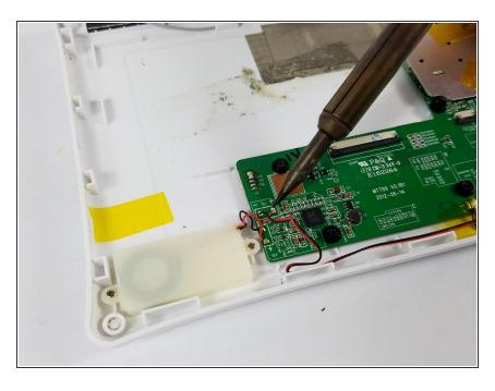
Using the soldering iron, detach the speaker's wires from the circuit board.
