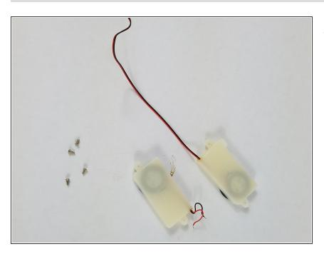
Once the screws have been removed, remove the speakers from the device.
