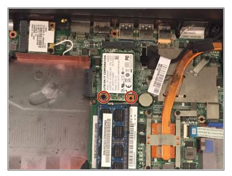
Use the #J1 Phillips Screwdriver to unscrew two 4 mm #J1 Phillips screws from side of the SSD drive closest to you.
