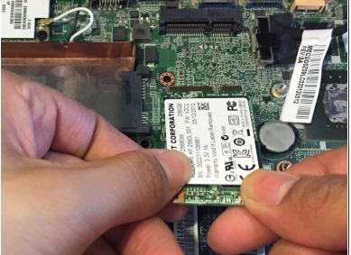
Gently lift up the SSD drive and pull it toward you to remove the drive fully from the laptop.
