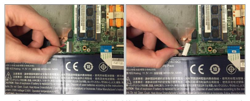
Gently disconnect the six bundled cables (red, black, and green) attached to both the battery and motherboard by pinching them with your thumb and forefinger. Pull with moderate force towards the left to disconnect.
