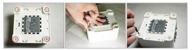
• Remove the four 7.5mm length Philips head screws under the rubber cover.
