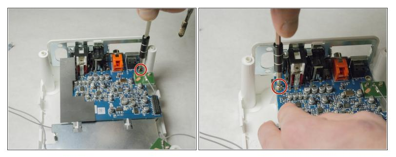
• Remove the two 7.5mm length screws on the top of the board.
