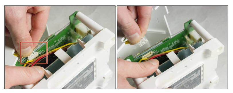
• Remove the connection for the front buttons to fully remove the cover.
