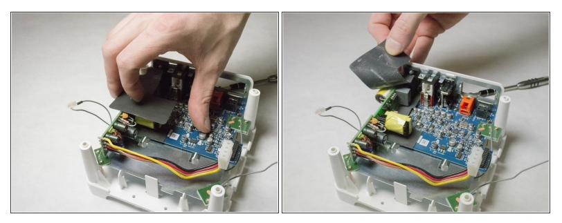
• Remove foam protective insulator from the bottom board.
