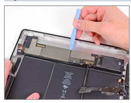
Use the edge of a plastic opening tool to gently pry the logic board up from the adhesive securing it to the rear case.
