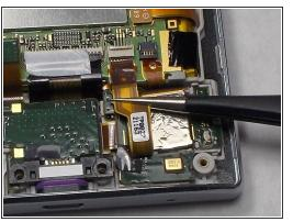
To disconnect the cable, use the tip of a spudger or your fingernail to flip up the small retaining flap. Then, you can safely pull the ribbon cable out.
