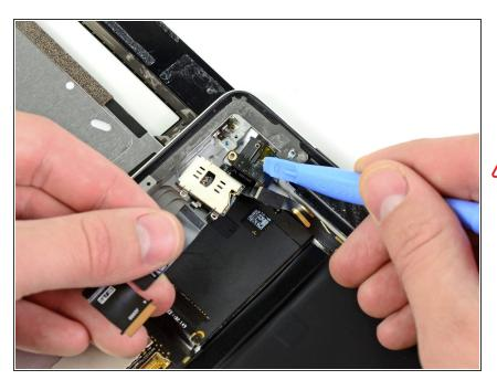
Use a plastic opening tool to help pull the headphone jack away from its recess in the top edge of the iPad.
