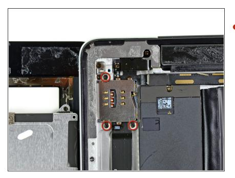
Remove the three 2 mm Phillips screws securing the SIM slot to the rear panel.
