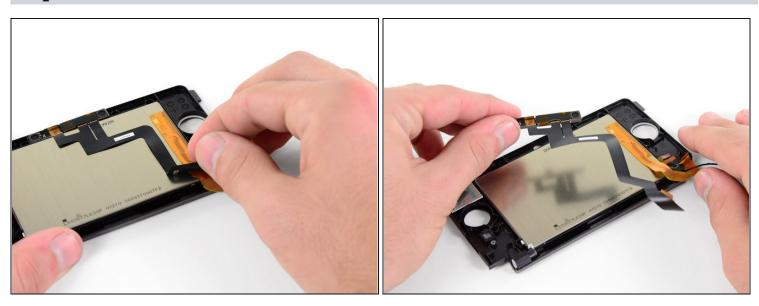
Peel the camera ribbon cable off the back of the upper LCD.
