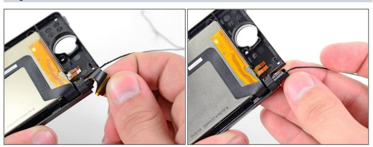
• Gently roll the upper LCD ribbon cable and camera ribbon cable together and insert them into the hinge opening.
