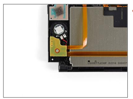
Remove the 2.5 mm Phillips screw securing the right speaker board to the upper display bezel.
