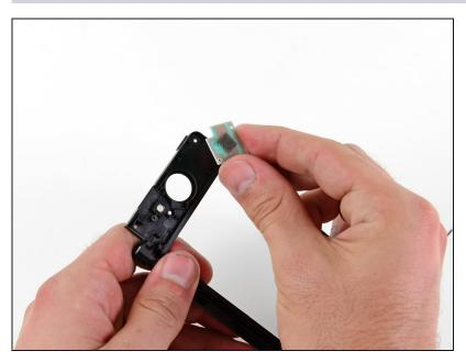
• Remove the Wi-Fi antenna from the upper display bezel.
