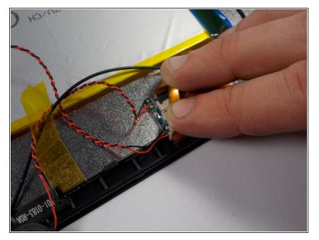
The two wires that connect the speakers to the motherboard must be removed next. In order to replace the speakers you will need to solder them back into place.
